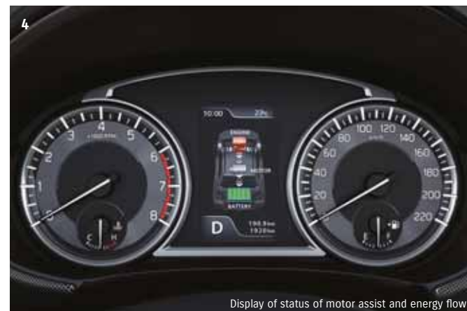
Display of status of motor assist and energy flow
